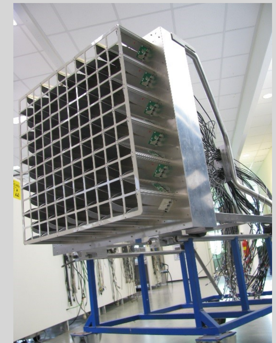
The FPA system obtained from ASTRON (Netherlands), which is being used to prototype the GMRT FPA; the 72-element Array Feed is shown in the right panel, and the FPA computing racks in the left panel.
