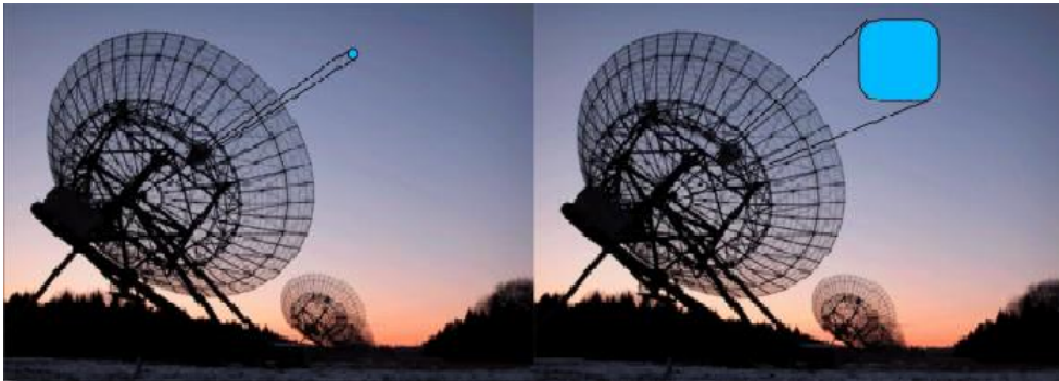
Figure 1.4: Difference between field of view with single receiver feed and Focal plane array feed
