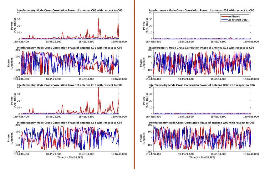
5 degrees off-source, shows correlated RFI, Filtering at 2 sigma threshold (replaced by zero), unfiltered in red color, filtered in blue color
