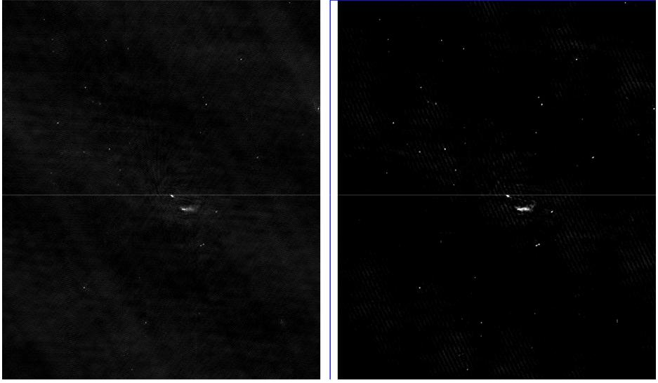
250-500 MHz, 16 antennas, Pol.-1 (left, without filter) & Pol.-2 (right, with broadband RFI filter), factor of two improvement post-filtering
