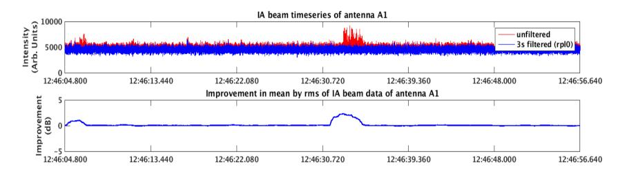
Single spectral channel (650 MHz) plot over time (Incoherent Array mode) at 1.3 ms time resolution for filtered and unfiltered outputs
