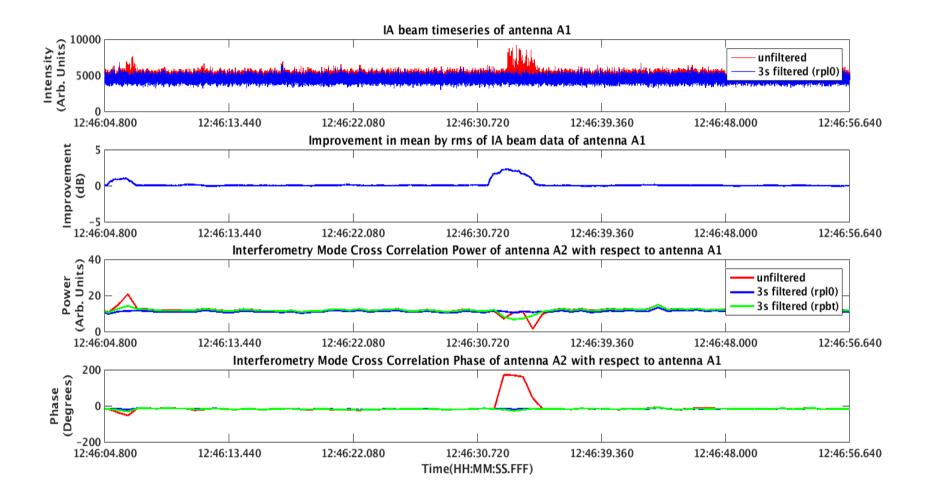
Beam and correlator output of a spectral channel showing filtering at 3σ threshold – replacement with zero and threshold
