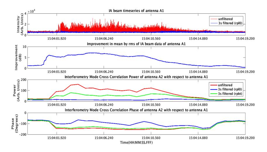
Beam and correlator data of a spectral channel showing filtering at 3**σ** threshold – replacement with zero and threshold
