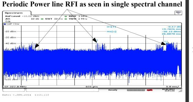
• The ITU-R RA.769-2 report [1] defines the level of RFI as detrimental when its presence introduces more than a 10% RMS error in the flux measurement.
