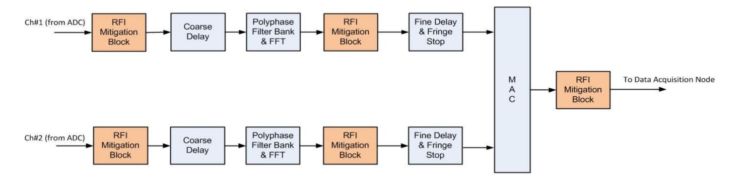
In order to remove diverse types of RFI, RFI Mitigation is proposed to be carried out in pre-correlation and postcorrelation domains in the digital subsystem of the GWB.
