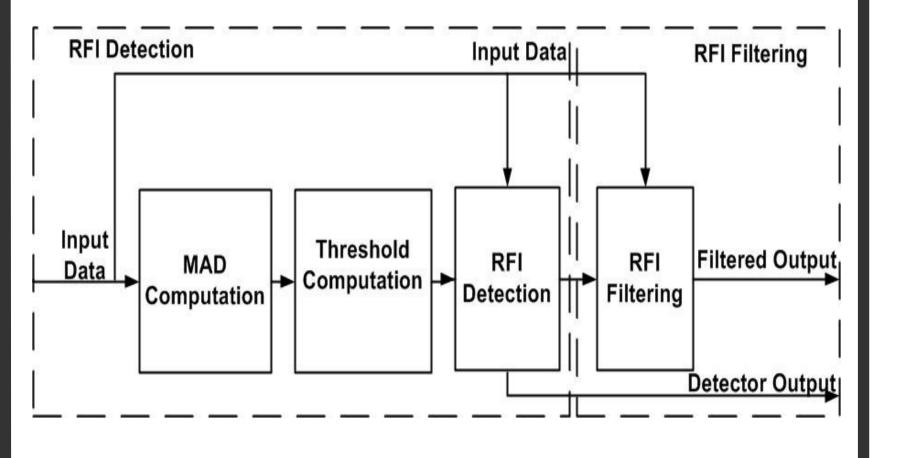
RFI mitigation block [3] was designed using MATLAB-Two RFI mitigation blocks each having 4K Simulink and Xilinx System Generator and implemented on ROACH-1 FPGA board designed by CASPER collaboration window size utilize 67% resources on Xilinx Virtex-5 SX95 FPGA. (https://casper.berkeley.edu/).
