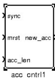
Figure 15: Accumulator Control Block
