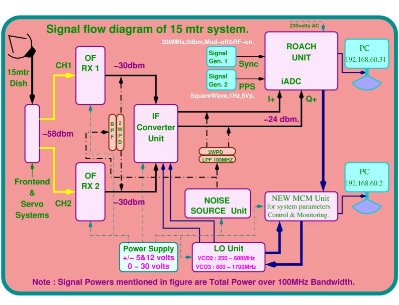
Analog signals from the 15 meter dish base , comes to 15mtr system in the lab through optical cable. After converted back to electrical, these signals reaches the digital backend through IF system.
