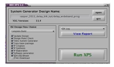
Make sure the file displayed in the pop-up is correct and then click the <i>Run XPS</i> button. After compilation, it creates a directory named after the model file name without the .mdl extension. There is a sub directory named bit\_files. In this bit\_files directory there are .bit and .bof file. We need the .bof file to program the FPGA.
