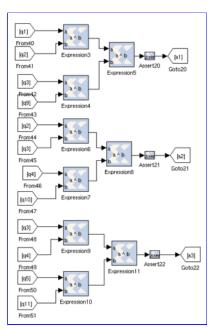
Concatenate the bits to get 4-bit output and also provide an input port for reset.
