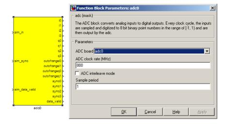
The first step to creating a frequency spectrum is to digitize the signal. This is done with an ADC – an Analogue to Digital Converter. In Simulink, the ADC daughter board is represented by a yellow block. Work through the "iADC tutorial" if you're not familiar with the iADC card.
