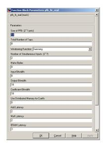
There are two main blocks required for a polyphase filter bank. The first is the **pfb\_fir\_real** block, which divides the signal into parallel 'taps' then applies finite impulse response filters (FIR). The output of this block is still a time-domain signal. When combined with the **FFT\_wideband\_real** block, this constitutes a polyphase filterbank.
