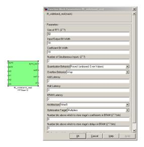
The **FFT\_wideband\_real** block is the most important part of the design to understand. The cool green of the FFT block hides the complex and confusing FFT butterfly biplex algorithms that are under the hood. You do need to have a working knowledge of it though, so I recommend reading Chapter 8 and Chapter 12 of Smith's free online DSP guide (at <a href="http://www.dspguide.com/">http://www.dspguide.com/</a>).
