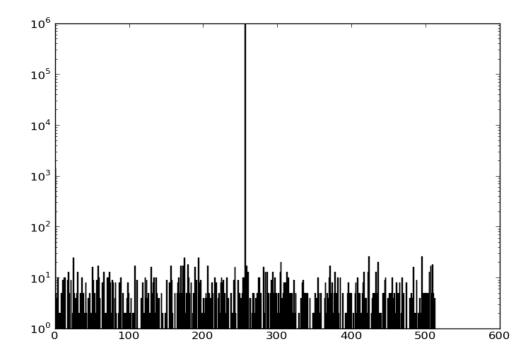
Each line of the recorded data file contains continuous real and imaginary data from the same channel. The data folder has a sample recording named channel256\_out that contains data recorded with a 200MHz tone feeding an iADC. Press Ctrl+c and then Enter in the terminal to stop this plot.
