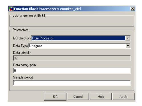
Note the field *Data bitwidth* is greyed out with a value 32. This is because all software registers have a fixed data bitwidth of 32 bits.
