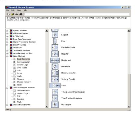
Double-click on the newly added slice block. There are multiple ways to select which bit(s) you want. In this case, I find it simplest to index from the upper end and select the first bit. If you wanted the lsb, you could also index from the lsb,. You can either select the width and offset, or two bit locations.
