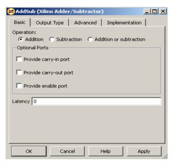
The output register is 32 bits. If we add two 32 bit numbers, we will have 33 bits. There are a number of ways of fixing this:
