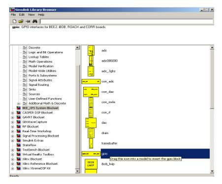
Set it to use ROACH's LED bank as output, GPIO bit index 0 (the first LED).
