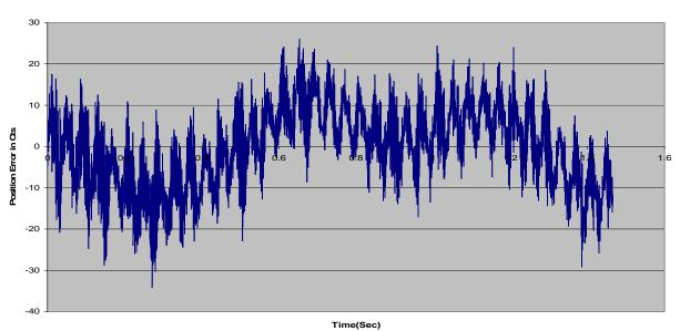
Position Error in Cts at Constant High Speeds (i522=10Cts/ms or 666 rpm)
