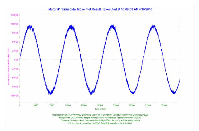
Figure 1 - Response to a Sine Wave input freq = 0.1 Hz given through pmac tuning pro
