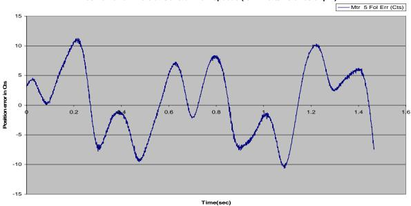
Position error in cts at Constant low speeds (i522=1cts/ms or 66.6 rpm)
