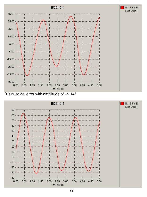
→ sinusoidal error with amplitude of +/- 24"
