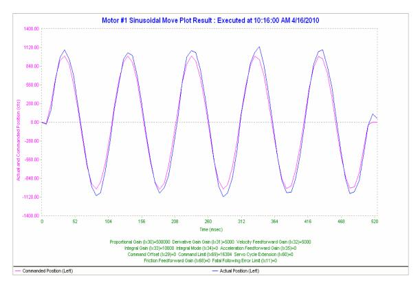
Figure 2 - Response to a Sine Wave input freq = 10 Hz given through pmac tuning pro Calculations of Magnitude and phase from each frequency response plots  $\mathbf{f} = \mathbf{10} \text{ Hz}$
