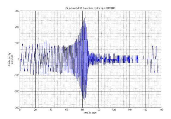
Resonance frequency: 1.33Hz, cut-off: about 1.5Hz
