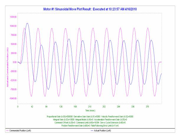
Figure 4 - Response to a Sine Wave input freq = 25 Hz given through pmac tuning pro Calculations of Magnitude and phase from each frequency response plots  $\mathbf{f} = \mathbf{25} \text{ Hz}$
