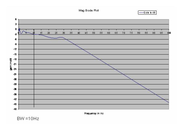
3 dB bandwidth of Velocity loop is given by **10Hz** (according to above fig.)
