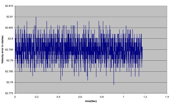
Velocity Error in Cts/sec with P9=63 and ADC=10V
