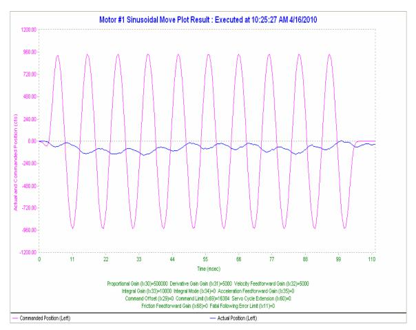
Figure 5 - Response to a Sine Wave input freq = 100 Hz given through pmac tuning pro
