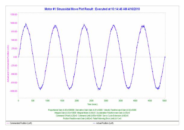
Figure 2 - Response to a Sine Wave input freq = 1 Hz given through pmac tuning pro
