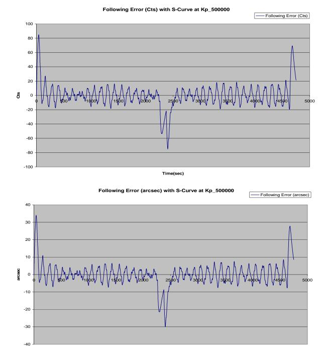
The following shows Channel #5 (Encoder) S Curve move plot with Kp=5, 00,000, Kd=10,000 Kvff=10,000, Ki=10,000
