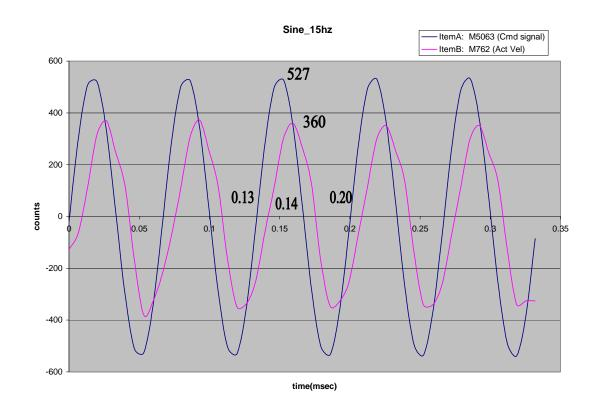
Calculations of Magnitude and phase from each frequency response plots f = 15 Hz
