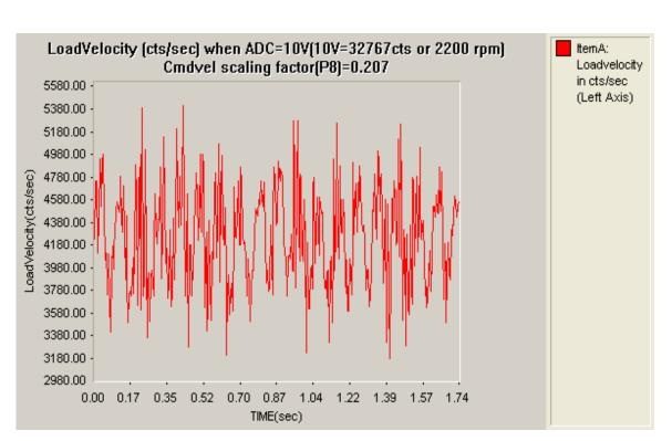
Loadvelocity in deg/min (Left Axis) when ADC=10V(10V=32767 or 2200 rpm) with Cmdvel Scaling factor(p8)=0.207
