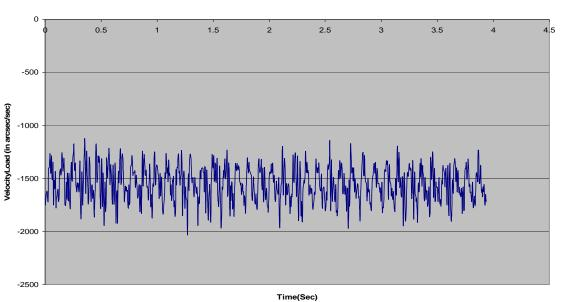
Load velocity plot for ADC=10V(10V=2200rpm or 32767cts) with Vel. Cmd Scale factor(P9=50)
