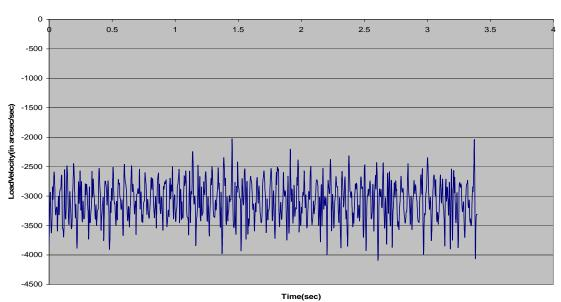
Load velocity plot for ADC=10V(10V=2200 rpm or 32767cts),CmdVel scale factor(P9)=100
