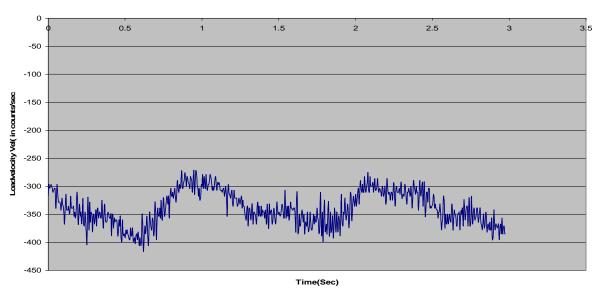
Load velocity plot for ADC=10V(10V=2200 in rpm) with Vel. Cmd scale factor(P9)=5.
