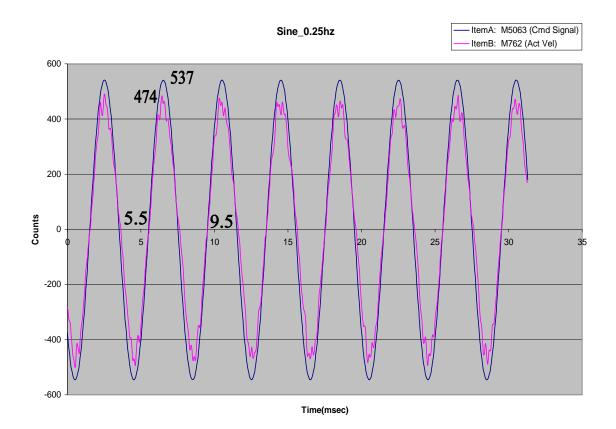
Calculations of Magnitude and phase from each frequency response plots f = 0.25Hz
