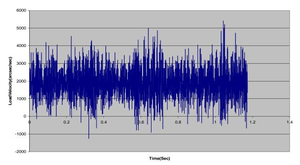
LoadVelocity (arcsec/Sec) with ADC=10V(10V=32767cts or 2200 rpm) and CmdVel Scaling factor (p9)=63
