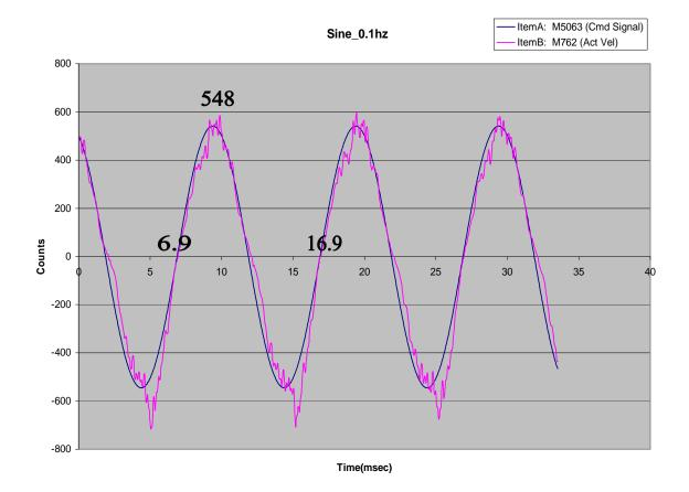
Calculations of Magnitude and phase from each frequency response plots f = 0.1Hz
