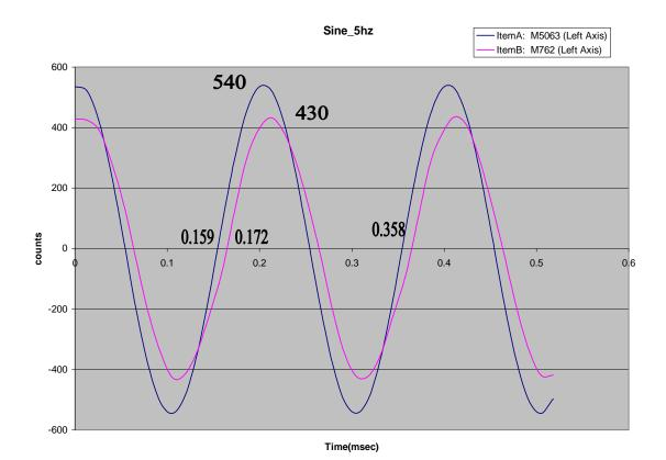
Calculations of Magnitude and phase from each frequency response plots f = 5 Hz
