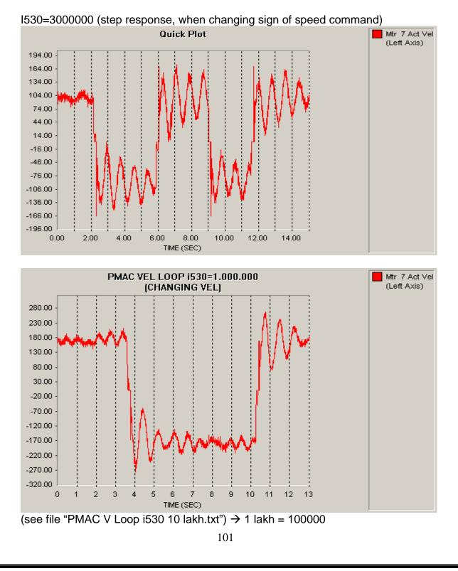
Check with low pass filtering the PID:  $\rightarrow$  100 Hz and 10 Hz (low pass 2. order), no changes
