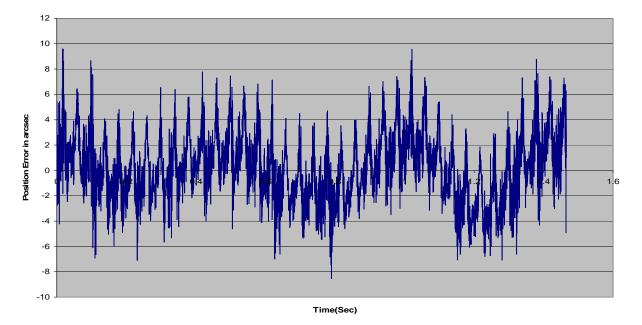
Position Error in arcsec with kp=4000000 and i522=10Cts/ms or 666rpm
