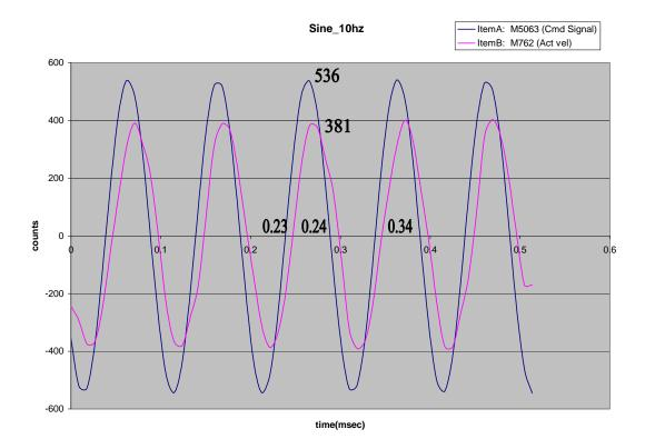
Calculations of Magnitude and phase from each frequency response plots f = 10 Hz
