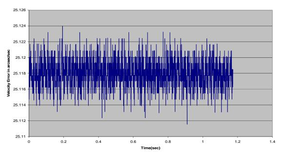
Velocity Error in arcsec/sec with P9=63 and ADC=10V
