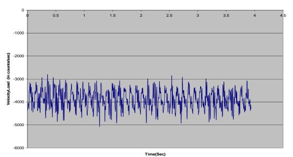
Load Velocity plot for ADC=10V(10V=2200 rpm or 32767cts), Vel.Cmd scale factor(P9)=50
