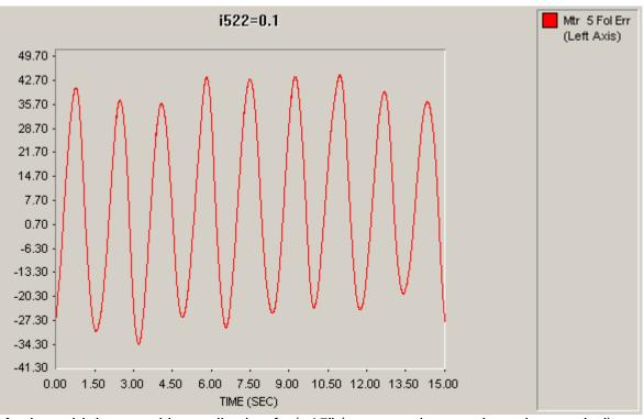
$\rightarrow$  sinusoidal error with amplitude of +/- 15" (measured over a long time period)
