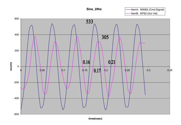
Calculations of Magnitude and phase from each frequency response plots f = 20 Hz
