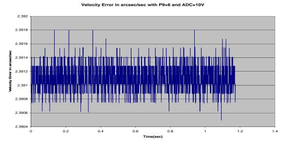
Velocity Error with P9 (Cmd Vel Scaling Factor) =6 and ADC=10V is **5.9** Cts/sec or **2.39** arcsec/sec.
