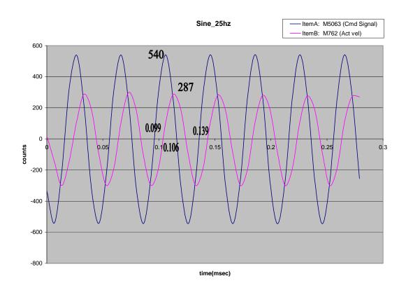
Calculations of Magnitude and phase from each frequency response plots f = 25 Hz
