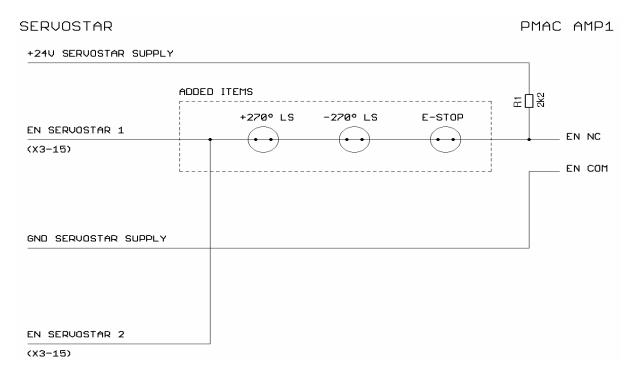
Circuitry of enable part (interconnection BLC and Servostar)
