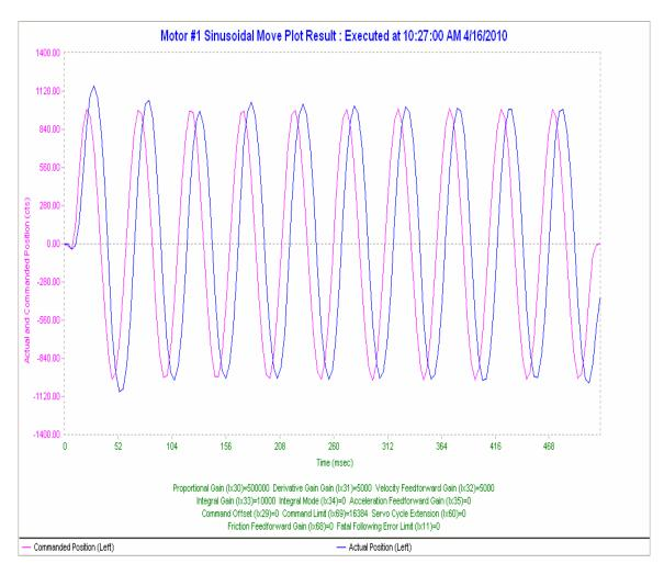
Figure 3 - Response to a Sine Wave input freq = 20 Hz given through pmac tuning pro Calculations of Magnitude and phase from each frequency response plots  $\mathbf{f} = 20$  Hz
