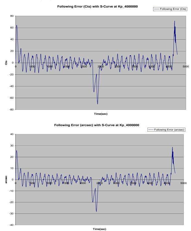
The following shows Channel #5 (Encoder) S Curve move plot with Kp=40, 00,000, Kd=10,000 Kvff=10,000, Ki=100,000
