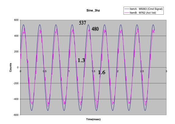
Calculations of Magnitude and phase from each frequency response plots f = 3 Hz
