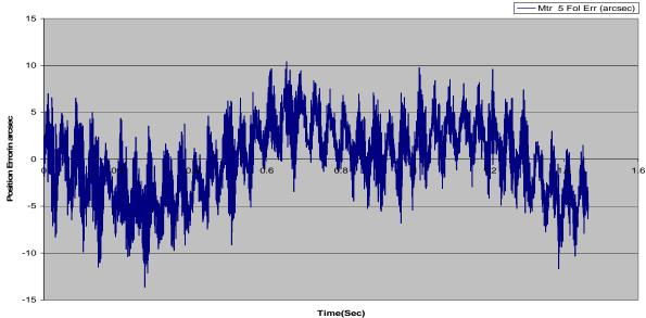
Position Error in arcsec at Constant High Speeds (i522=10Cts/ms or 666 rpm)
