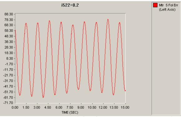
$\rightarrow$  sinusoidal error with amplitude of +/- 26" (measured over a long time period)
