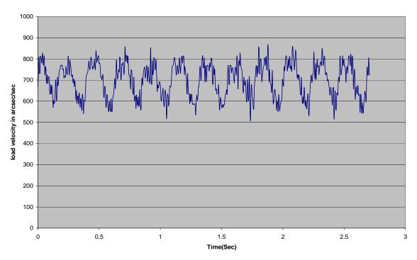
Load Velocity scaled and plotted in arc second / second for the same analog I/p of 1V
