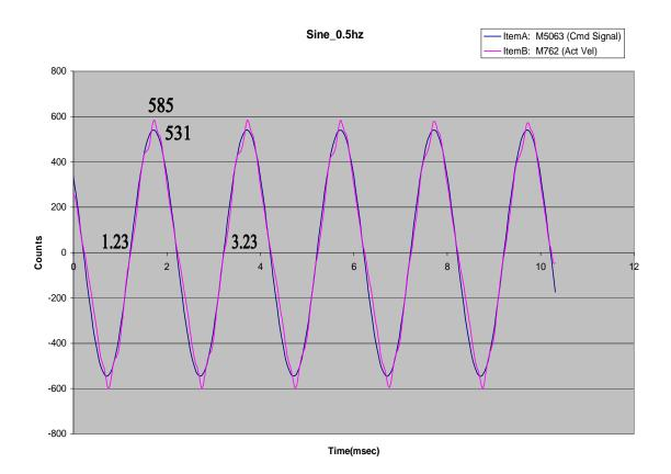
Calculations of Magnitude and phase from each frequency response plots f = 0.5Hz
