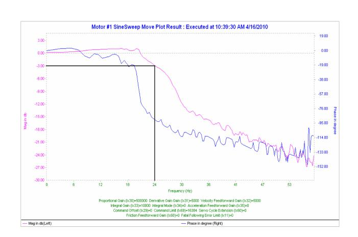
The Bandwidth of Position Loop according above Sine Sweep Bode Plot is 24 Hz The Resonant peak is approximately 1 dB and resonant frequency is 20Hz.
