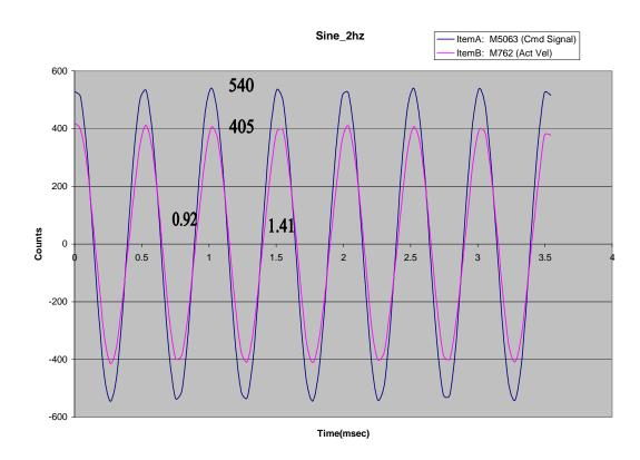
Calculations of Magnitude and phase from each frequency response plots f = 2 Hz
